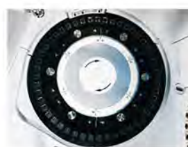
Reaction Tray 37±0.1°C, real-time monitor.
