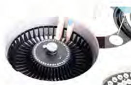
Reagent Tray 2~8°C cooling for 24 hours.
