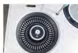
Reaction Tray 37±0.1°C, real-time monitor.
