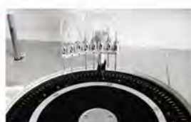
Washing Probe Independent 7-step washing system.
