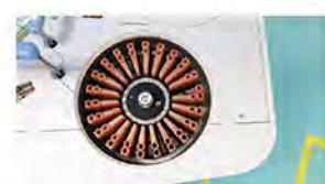
Reagent Tray 2~8°C cooling for 24 hours
