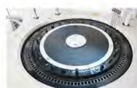
Reaction Tray 37±0.1°C, real-time monitor.
