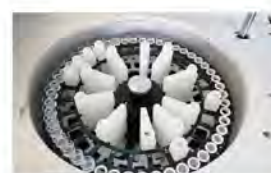
Reagent Tray 2~8°C cooling for 24 hours.
