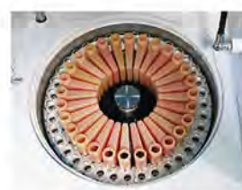
Reagent Tray Refrigerated tray with independent switch.
