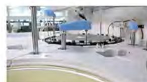
Mixer Probe Dual mixer, auto frequency adjustment
