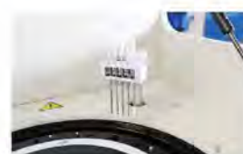
Washing Probe Independent 4-step washing system.
